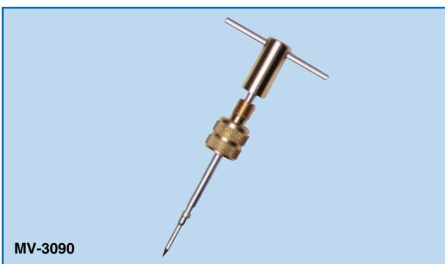
**MV-3090** Punches a hole in copper tubing through a "V-SERIES" fitting for the installation of a core without loss of gas (see page 111).
